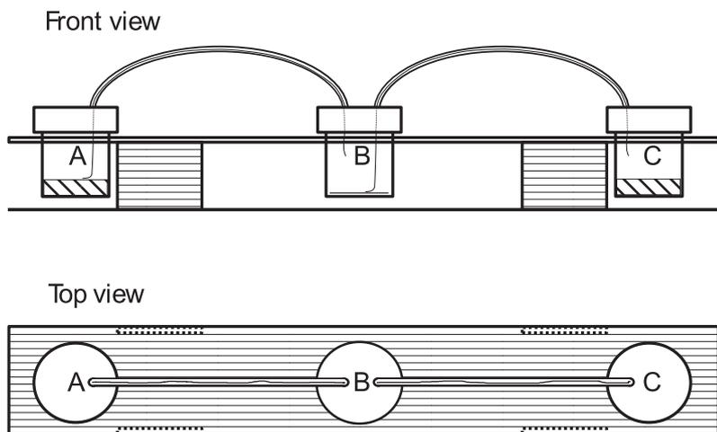
**Figure 2** Example schematic of design 3. Front and top views of the plywood housing for maintaining structure and consistency of the tubing insertion angle and tubing length for the dispersal apparatuses.
